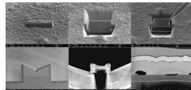
Figure 2: Secondary electron images of FIB sample preparation of an electron transparent section of a chalcogenide multilayer solar cell deposited by a novel deposition process for subsequent TEM analysis (sample provided N. Gaillard, Hawaii Natural Energy Institute (HNEI)).
