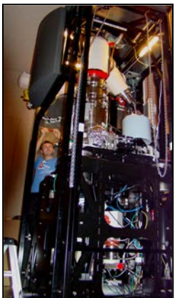
80-300 keV mono-chromated & dual Cs-corrected Titan "SuperSTEM" at U. Hawaii
