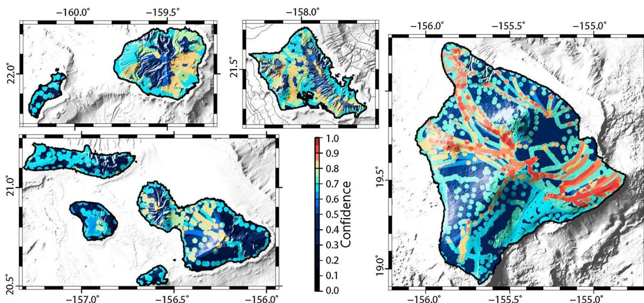
Fig. 2. Results of the Phase 1 geothermal play fairway confidence analysis for the State of Hawaii. Color indicates confidence in the probability values shown in Fig. 1. Confidence is a function of the number and quality of datasets at each location as well as their relative weight on influencing probability.
