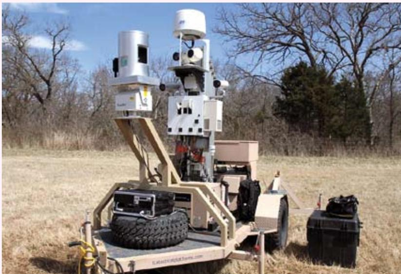
**Hyperspectral imagers remotely gather data from across the electromagnetic spectrum to identify chemical signatures of things, such as weapons in the landscape, the human eye doesn't detect**
